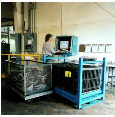
Precision parts are coated in one of Parker's rack lines using custom tooling designed for each job.
