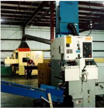
Two of the circular saws at the new plant. Precision cutting of all types of metal bar stock is available for diameters up to 14 inches.
